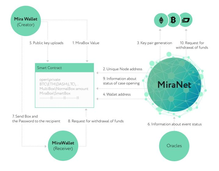
1. User initiates (Smart) MiraBox creation in an application (Desktop/Web/Mobile) and configures conditions for when the Box can be opened. In addition, the smart contract responsible for a particular box is deployed, and at this time a user is charged in MRC.
